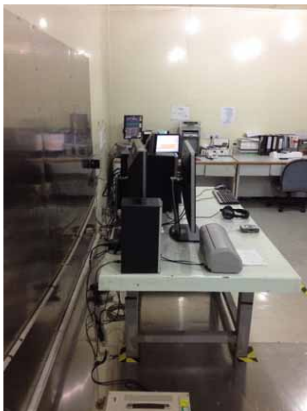
Side View of Conducted Emission Measurement (Telecommunication port)
