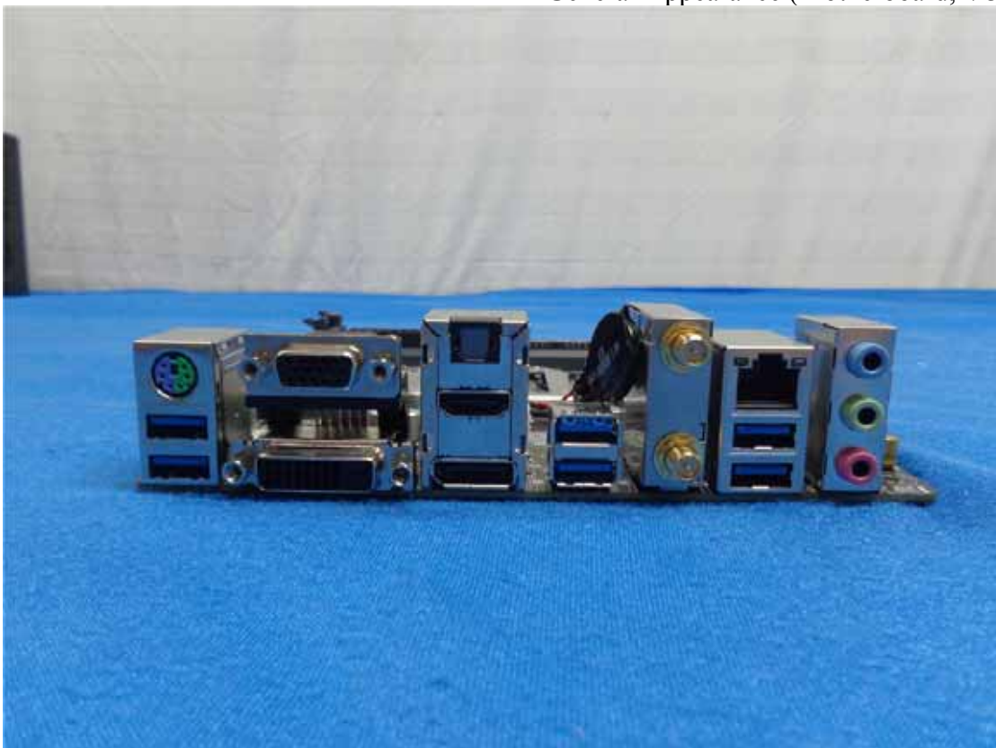
Figure 6 General Appearance (Motherboard, I/O Ports)
