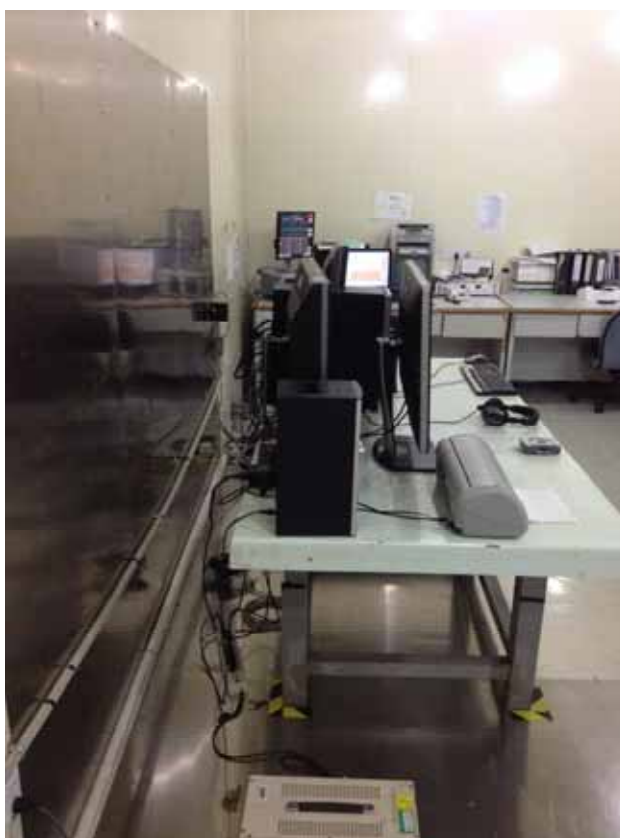
Side View of Conducted Measurement (AC Mains Port)
