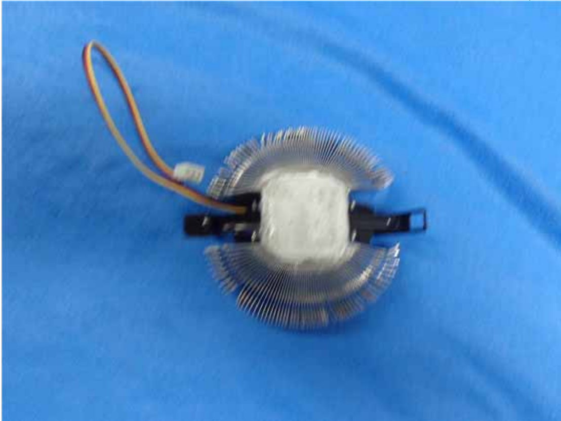
Figure 5 Fan Set(Back View)
