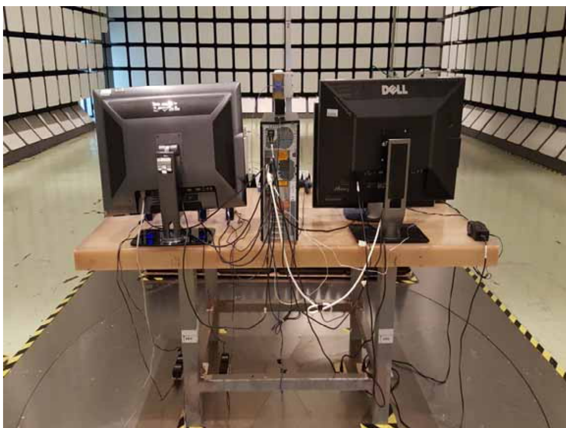
Back View of Radiated Disturbance Measurement
