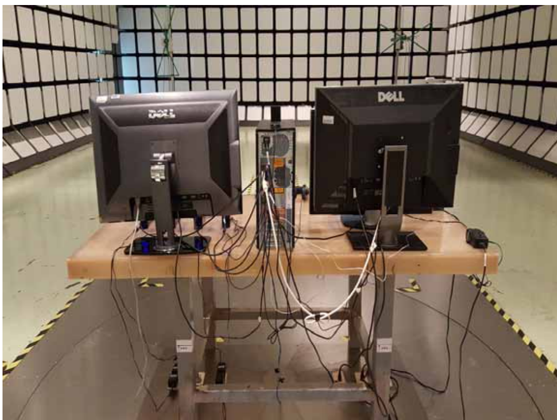
Back View of Radiated Disturbance Measurement
