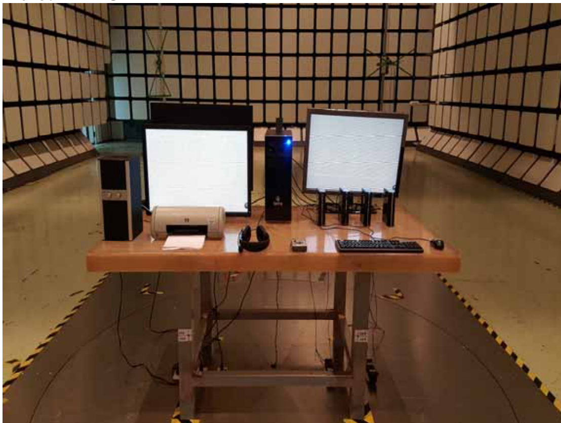
Front View of Radiated Disturbance Measurement
